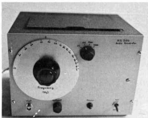
fig. 2. New HO-200 audio oscillator uses readily available parts.
